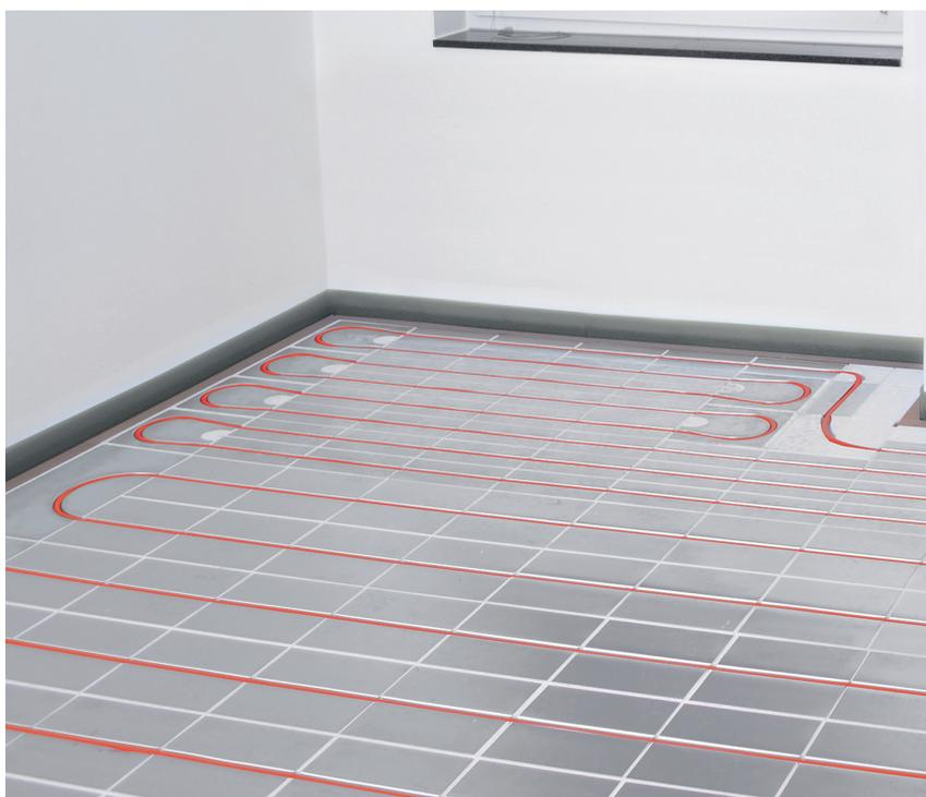
You can see the area with the finished Proline ENERGY BasicLine installation in the image above. The PROSECUREfibretec 2.0 is bonded over the entire surface with PROFIX dispersion fixative to protect the laid elements and the pipe as well as to stabilise the surface. The following installation steps can be found in our system configurations.
