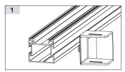
Insert the PROSTILTadvance 2.0 cross connector into the C-groove of the base profile as shown in the drawing (image 1) and rotate clockwise by 90 degrees.
