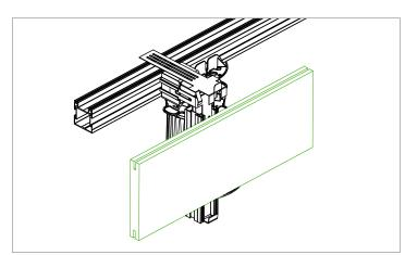
Once all edge profile brackets are positioned on the base profile with connection brackets, the first facing board can be inserted in the start and end holder.
