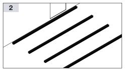
We recommend preparation of all longitudinal profiles to start with. For this purpose, shorten the base profiles to the desired length, or attach additional base profiles with the PROSTILTadvance 2.0 Connector L (see below "Profile connections")
