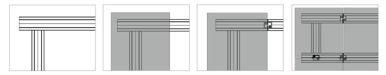
First row of slabs: If the first row of slabs is not secured against slipping with edging like the PROSTILTadvance stop clip X, we recommend to attach the slabs to the substructure with suitable mounting adhesive.
