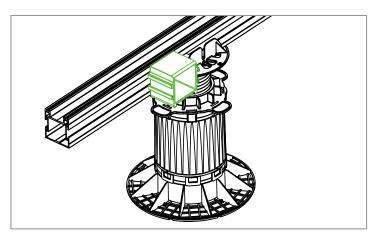
Insert the PROSTILTadvance 2.0 edge profile bracket into the lateral C-groove of the base profile (same procedure as for the cross connector) and move into the desired position. It must be ensured that when using profiles without silence strip, the smooth side of the edge profile bracket is flush at the top with the base profile.
