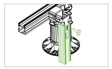
A base profile piece, which is cut to size, can now be screwed to the holding strip of the connection bracket pointing down, using the drilling screws as shown in the drawing.
