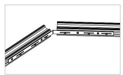
The connector can now be screwed onto the adjacent base profile as shown in image 4.
