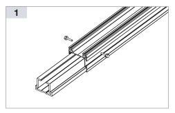
To connect the base profiles in the length, the PROSTILTadvance 2.0 Connector L is required. For this, the Connector L is inserted into the profile opening on the head side of the base profile up to about half, as shown in image 1.
