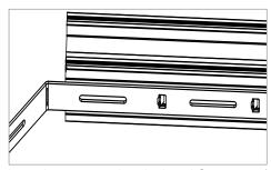
Insert the connector into the lateral C-grooves of the base profiles. Make sure that the guide lugs bent open in advance engage with the C-groove of the base profile.
