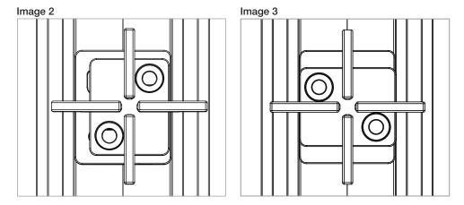
The cross joint can be inserted into the base plate in two positions.
