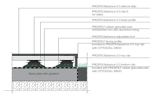
The edging of free laying a reas with a vertical facing slab is carried out using the PROSTILTadvance Clip U and the PROSTILT edge profile. For this purpose, the facing slab is to be cut from the surface covering material at the corresponding height, and positioned in the PROSTILT edge profile. The top edge of the facing slab is inserted into the bracket of the PROSTILTadvance Clip U, which is then screwed to the groove of the PROSTILTadvance base profile using stainless steel screws.
