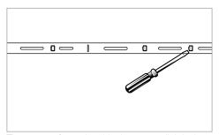
The pre-perforated guide lugs are slightly bent open by means of a slotted screwdriver.
