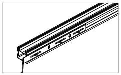
Image 6 If required, the position of the connector can be varied by loosening the drilling screws in the elongated hole.
