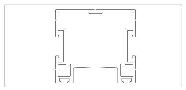
For the visible screw connection, e.g. for floorboards without groove, we recommend the profile alignment shown.
