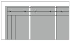
Lay the first board in the centre and attach to each longitudinal profile with two screws (1x ending profile, 1x longitudinal profile). Lay further boards and attach with two screws per longitudinal profile. Ensure a joint distance of approx. 7 mm here.
