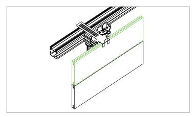
If more facing boards are required for the planned facing, they can be screwed in the joint area with the PROSTILTadvance 2.0 clip T to the rising base profile. The top facing board is held up with the retaining clips. Once the facing is properly positioned and aligned, tighten the loosely tightened screws in the elongated holes of the clip at the top.
