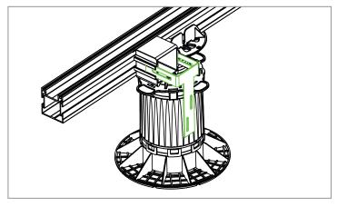
The connection bracket vertical L can be moved to the desired position by moving it in the C-groove of the edge profile bracket.
