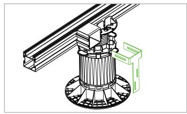
The connection bracket vertical  ${\sf L}$  can now be inserted in the C-grooves of the edge profile bracket.
