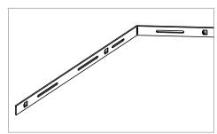
Manually bend the connector in the middle approx. to the mitre angle that is required.
