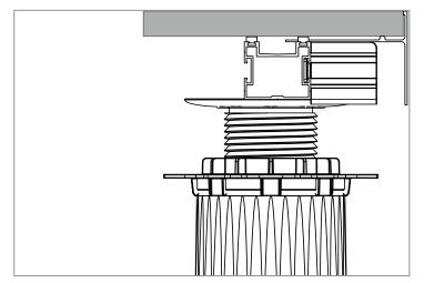
Our PROSTILTadvance 2.0 TOS-T-profiles can also be used as facing for ceramic and natural stone slabs up to 20 mm.
