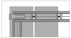
Now position the next board and screw it tight with more clips T. A joint distance of approx. 7 mm is automatically achieved with clip T.
