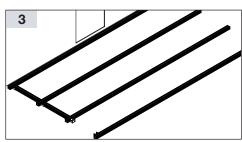
the base profiles for this purpose and install the PROSTILTadvance 2.0 cross connector at the correct distance (see p. 2 Track width).
