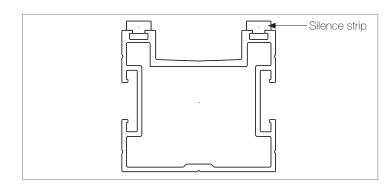
The silence strip is strongly recommended for minimising impact sound and prevention of cracking noises under slabs made of e.g. ceramic, natural stone or artificial stone.
