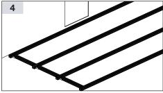
If required, additional cross connections can be inserted into the frame construction. The frame construction can now be placed on support pads or pedestal supports and aligned.
