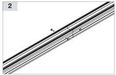
The Connector L is fixed in the C-grooves of the base profile with 2 drilling screws (6 KT flange  $4.2 \times 16 \text{ mm}$  item no. 94338).
