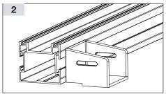
The cross connector can be inserted in any place in the C-groove. The cross connector can also be moved in the C-groove when inserted.
