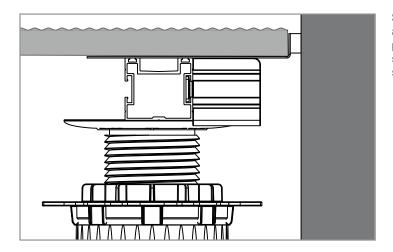
Spacers with neoprene pad must be installed to hold the last row of boards against the walls of buildings or towering components. The spacer is positioned on the edge profile bracket as shown in the drawing and then screwed tight. The edge profile bracket must be rotated so that the smooth side of the edge profile bracket are flush with the top edge of the base profile.
