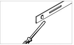
Use the screwdriver tip to engage in the small slotted holes of the connector and pry open the guide lugs.
