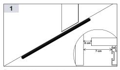
For patios joining onto the house, we recommend laying the first profile strut along the house wall. The correct distance to the house wall must be ensured (total of 7 cm: ground overhang approx. 5 cm distance to wall at least 2 cm)
