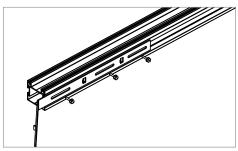
Fix the connector to the elongated holes by means of the drilling screw (6 KT flange 4.2 x16 mm item no. 94338).
