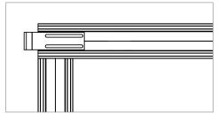
If required, insert the start and end holder in the profile, adjust it in the correct position and screw it tight with the drilling screw (6 KT flange  $4.2\,\mathrm{x}$  16 mm item no. 94338).
