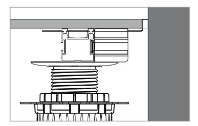
Spacers with neoprene pad must be installed to hold the last row of slabs against the walls of buildings or towering components. The spacer is positioned on the edge profile bracket as shown in the drawing and then screwed tight. The edge profile bracket must be rotated so that the lateral elevations of the edge profile bracket are flush with the silence strip of the base profile.
