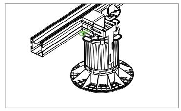
Fix the connection bracket vertical L using the drilling screw (6 KT flange  $4.2 \times 16$  mm item no. 94338) through the elongated holes of the holder.
