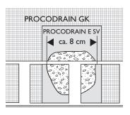
outside areas (at least C2F S1) approx, every 50 cm in lump form under the profile strip and over the PROCODRAIN E SV and fix the profile in it once it has been aligned. If necessary, use plastic shims or tile strips to support the height. The lumps should have a diameter of approx. 8 cm and enclose the T in the profile strip. The mortar escaping upwards should be scraped off with deep channels so that the following coarse grain mortar can take a hold in them.
